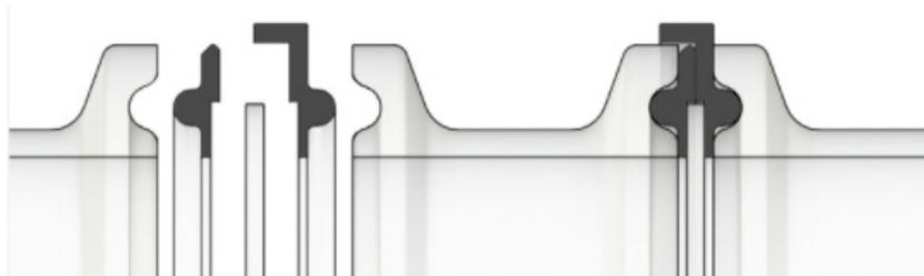
If we want to install an orifice plate with a thickness of 1,00 mm we use the above setup with two mating parts with both a 0,50 mm chamber. These two chambers total up to 1,00 mm. Carefully locate the center chamber and place the orifice plate inside and click the two gasket chambers together so they lock. Ready to use.
